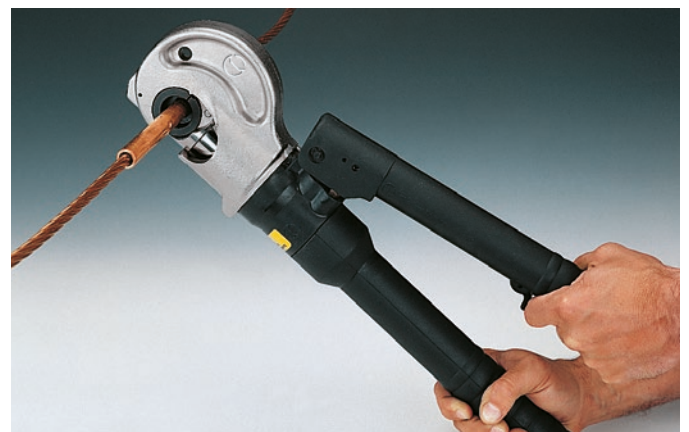
Die release system, protected from accidental operation
